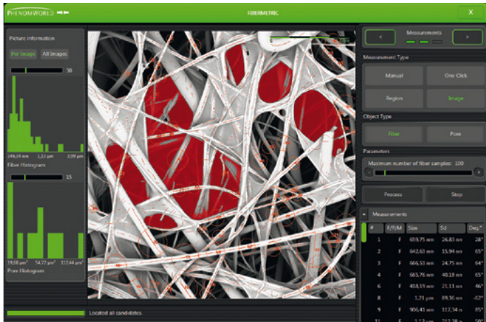
FiberMetric user interface with fiber and pore measurements
