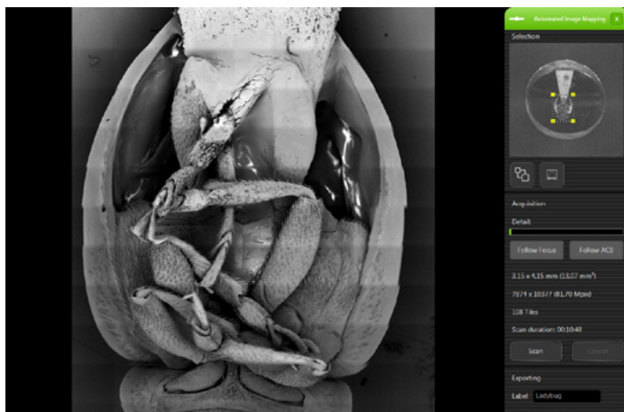
Example of large field of view automated image collection. The sample is a 3.15 x 4.15 mm ladybug that can be imaged completely at high resolution
